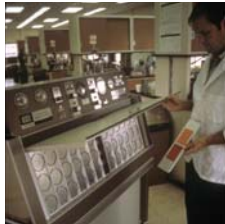
UV fluorescent weathering device used for accelerated testing.
